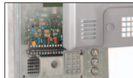
stainless steel plate and anti-vandal features protects all internal parts
